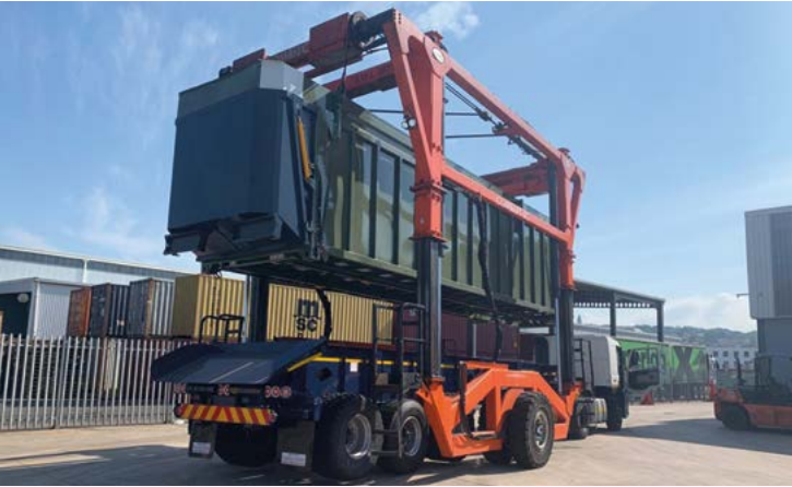
AZP-60 body mounted to the chassis
