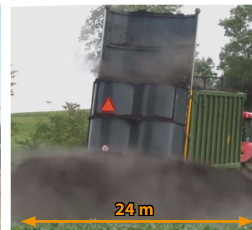
Defecate spread with plates. Closed tailgate
