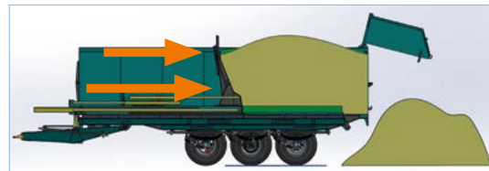
Half of bottom moves with front wall
