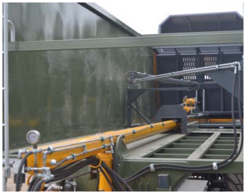
Hydraulic system of movable wall
