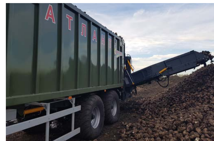
Beet piler up to a height of 3.0 m.
