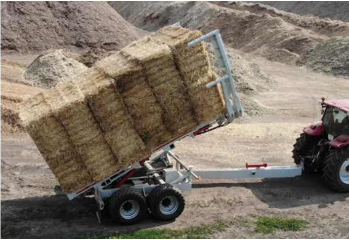
Unloading the bale semi-trailer on a flat and solid surface takes 30-40 seconds
