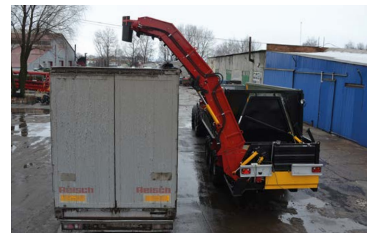
Beet reloader up to a height of 4.5 m.
