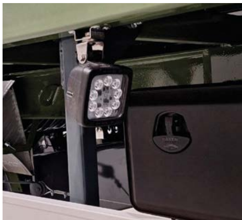
Side and back LED lights to illuminate the technological track on the field
