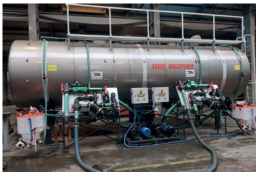
Stationary mortar unit RZS-20 with two independent compartments
