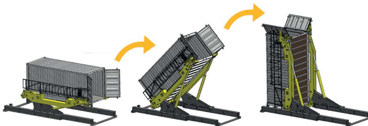
Container tipping process
