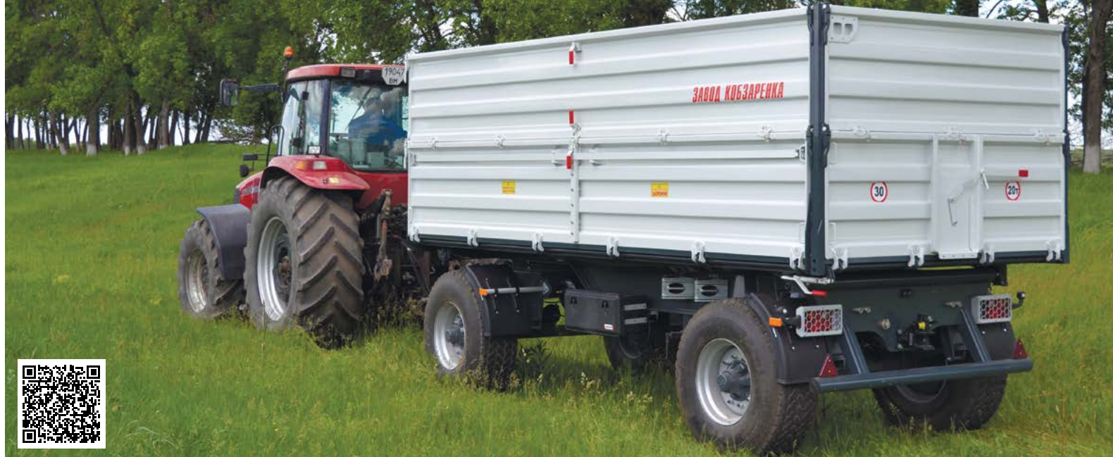
Three-way unloading trailers can be easily transformed into a conventional platform
