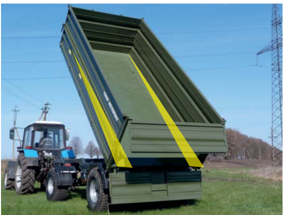
Conical body prevents of hanging green mass and fertilizers
