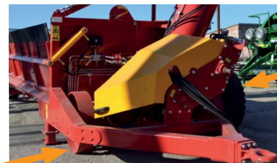
Additional front wheels option for transporting grain in hopper of BNP machine
