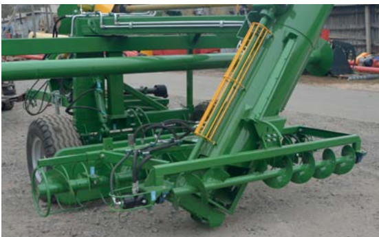
Additional horizontal auger for corn
