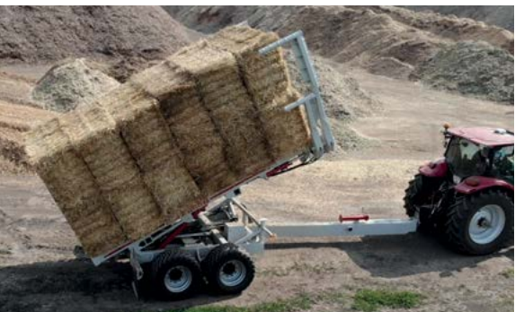
Unloading the bale semi-trailer on a flat and solid surface takes 30-40 seconds
