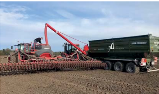
ShRP extension screw for loading seeders
