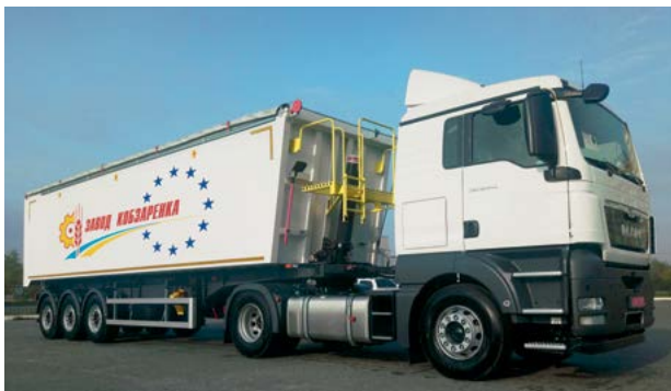
Aluminum Tipper Semi Trailer. Model 50, 55, 90 m 3
