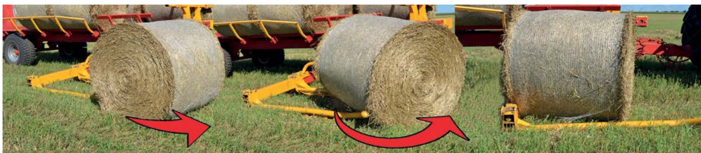
The universal hydraulic paw on the go unfolds the roll and loads on the platform
