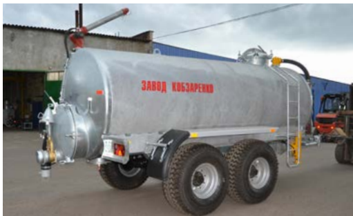
Hot dip galvanizing. Galvanizing layer 100-300 microns
