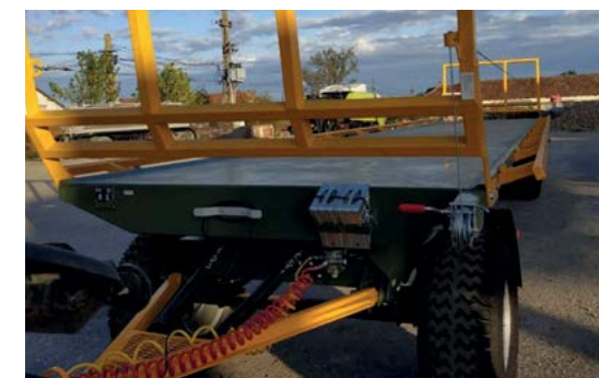
Winch and broadening of platform to 3 m
