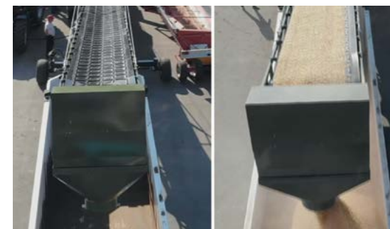
The V-shaped chevron belt 1,200 mm does not damage the seeds
