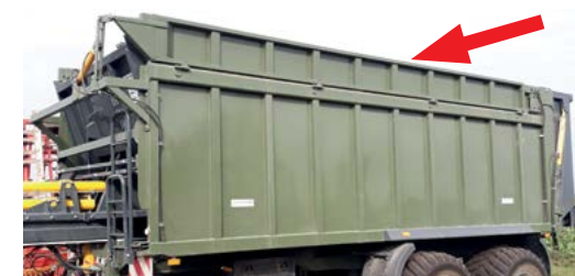
Hydraulic side opening h-400 mm
