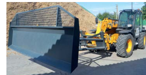
Extension for a telescopic loader for hilling grain, silage, wood chips, snow
