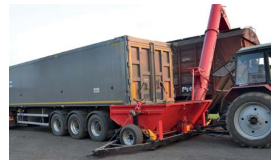
BNP-3 on the loading of the wagon parallel to the wagon
