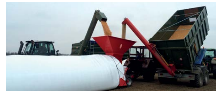
Hydraulically-folding auger GRSH-300/4,5
