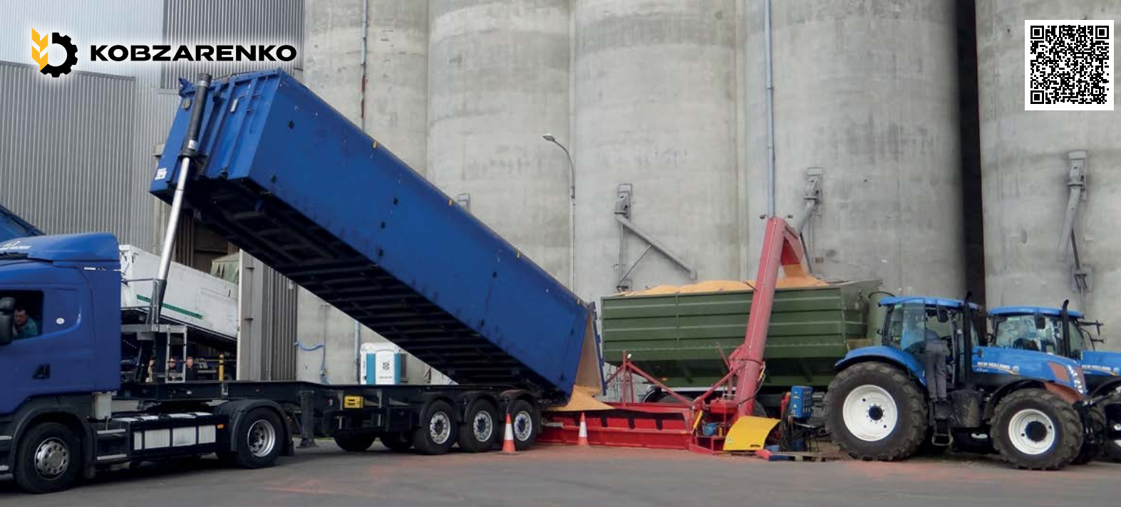
BNP-3 on the loading of the wagon parallel to the wagon
