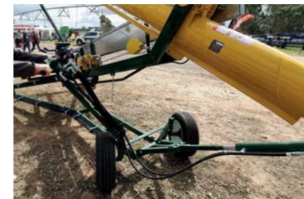
Additional option: rear wheels turning mechanism
