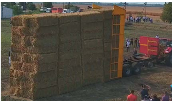
Unloaded bales in haystack without using of additional equipment
