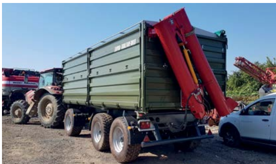
Back wall adopted for reloading auger
