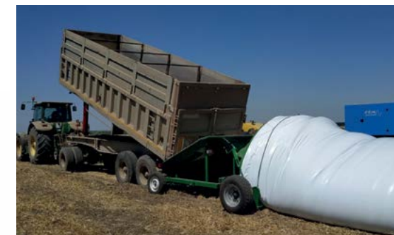
ZPM (A) -180 with a lowered hopper and an electric motor. Loading from a car.
