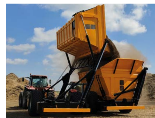
The maximum unloading height is 4,000 mm
