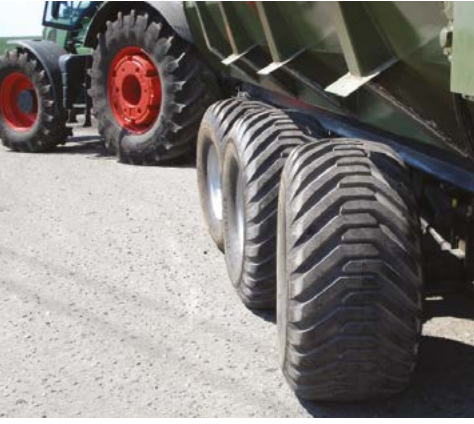
First and last axles are positively steered
