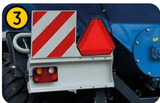
Road lighting of the trailer according to EU standards
