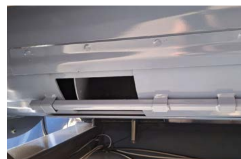
Three cleaning flaps of horizontal auger
