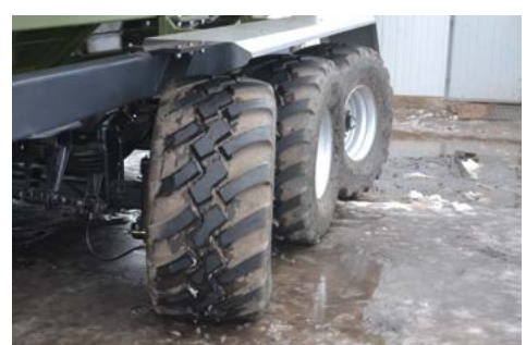
A hydraulically steering first and last axles (PBN-40 and PBN-50).
