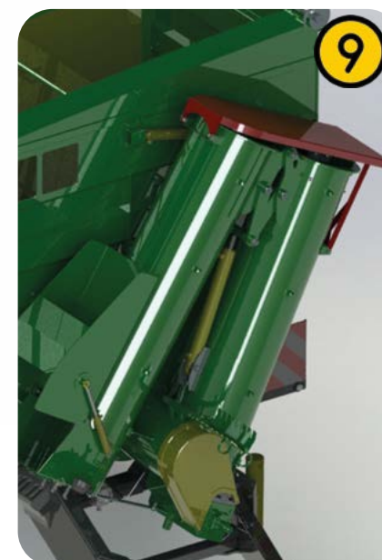
Protective cover of the auger against precipitation
