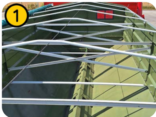
The sides of the body are pulled together by powerful profile spacers
