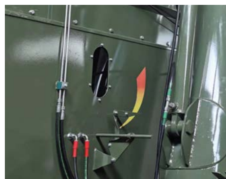
Indicator of slide gate opening
