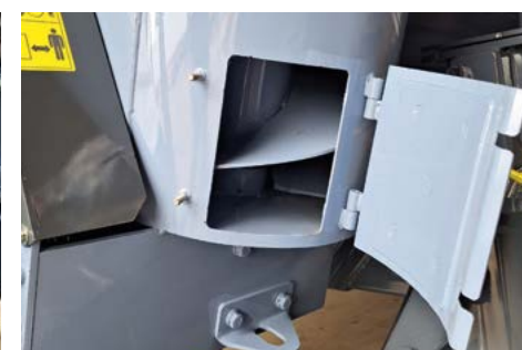
One hatch for cleaning of vertical auger
