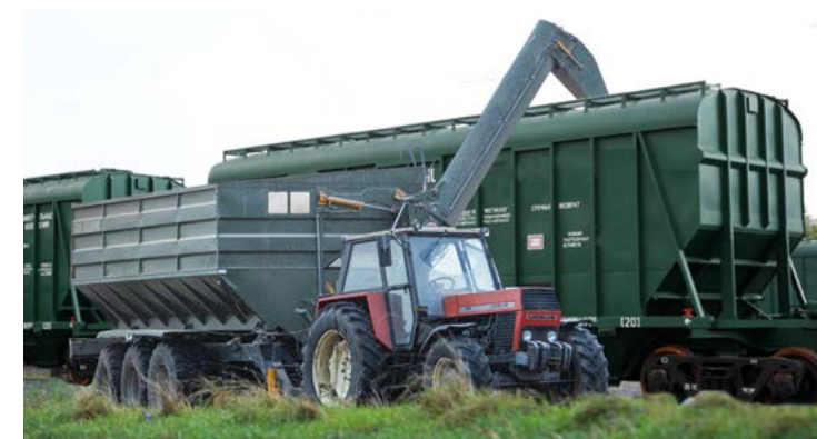
Extended auger h-5.5 m for loading wagons
