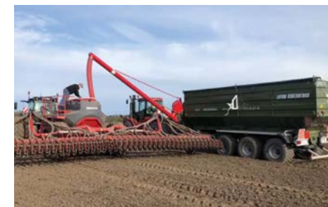
Loading of seeding machines through PVC hose
